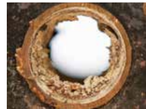
Unprotected tankless: Failed at 5.8 simulated years and 136,000 gallons
