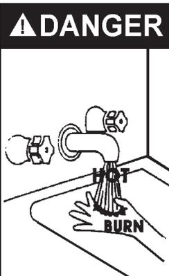
**▲ DANGER** Water temperature over 125°F (52°C) can cause severe burns instantly resulting in severe injury or death.
